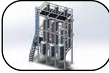
降膜浓缩系统 Falling Film Evaporator
